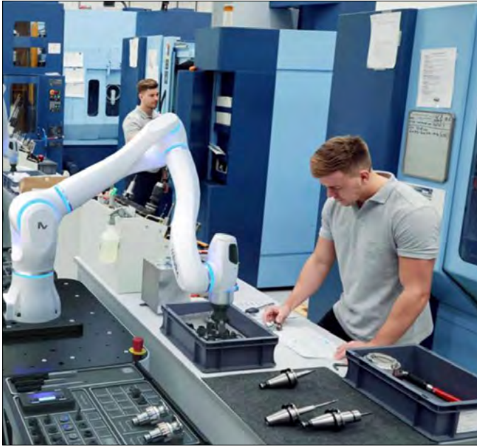
Pick & place s kognitivnim robotom MAiRA – Neura Robotics
